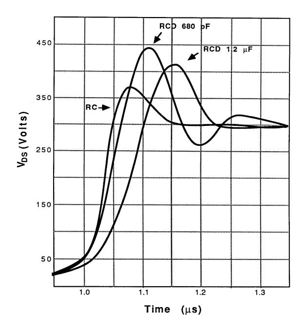
a combination snubber, using both RC and RCD, can produce very good results with low losses. An example of such a combination is given in figure 12 and the resulting waveform is compared to the previous RC snubber, using the same circuit conditions, in figure 13.
