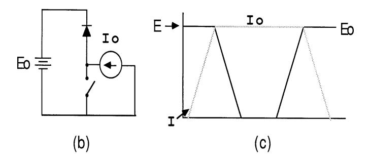
current in the diode, the switch voltage will remain at  $E_0$ . Once all of the current has been transferred to the switch, the switch voltage can begin to fall. At turn-off the situation is reversed. As the switch turns off, the voltage across it will rise. The current in the switch will however, not begin to fall until the switch voltage reaches  $E_0$  because the diode will be reverse biased until that point. Once the diode begins to conduct the current in the switch can fall.
