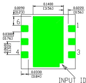
**Figure 1** Bottom side (foot print) of WHM25-1525AE
