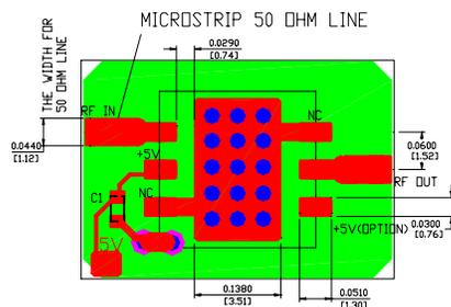
**Figure 2** Test board layout for WHM25-1525AE
