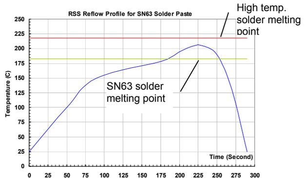
Figure 6 Recommended RSS solder reflow temperature profile.
