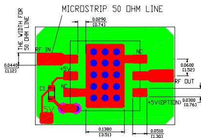
**Figure 2** Test board layout for WHM25-1525AE
