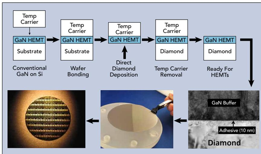
▲ Fig. 1 GaN on Diamond wafer process.
