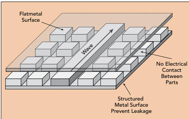
▲ Fig. 12 GAP waveguide structure.
