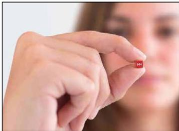
▲ **Fig. 9** The CUBE mXTEND™ antenna booster from Fractus Antennas (5 mm<sup>3</sup>).
