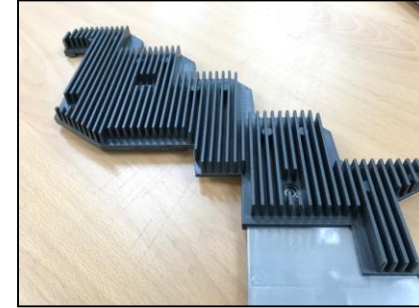
Thermal plastic heat sink(15W/mK)
