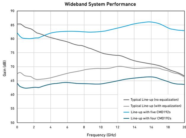
Figure 5. Overall system performance including equalization.
