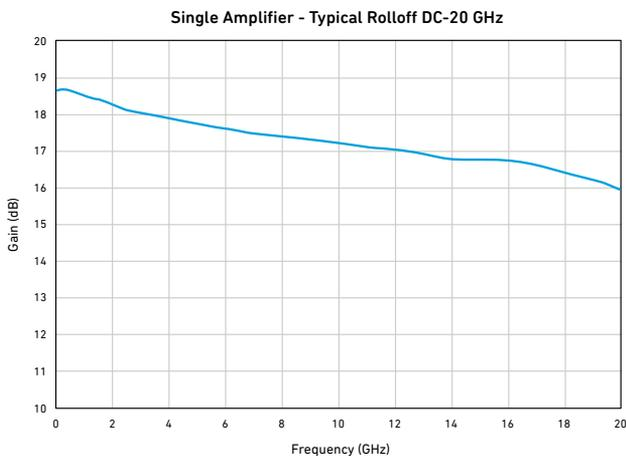
Figure 1. Frequency response of a typical distributed amplifier.
