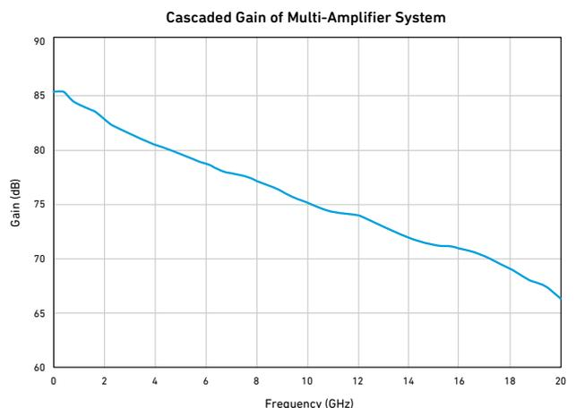
Figure 2. Frequency response of a typical wideband lineup.
