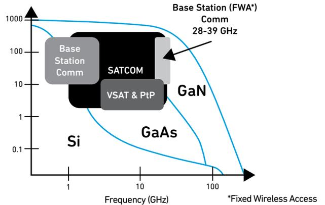
Figure 2. Suitability of semiconductor technologies to different applications.
