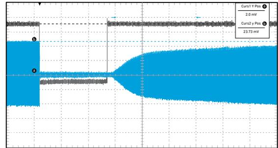
Figure 2. Typical oscilloscope trace for the measurement of pulse recovery time. Desired signal in blue, interferer pulse in magenta.
