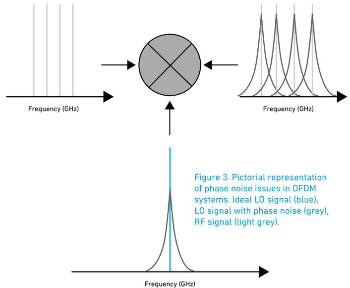
Figure 3. Pictorial representation of phase noise issues in OFDM systems. Ideal LO signal (blue), LO signal with phase noise (grey), RF signal (light grey).
