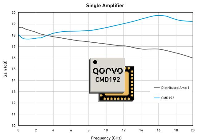
Figure 4. CMD192 vs. a typical distributed amplifier.
