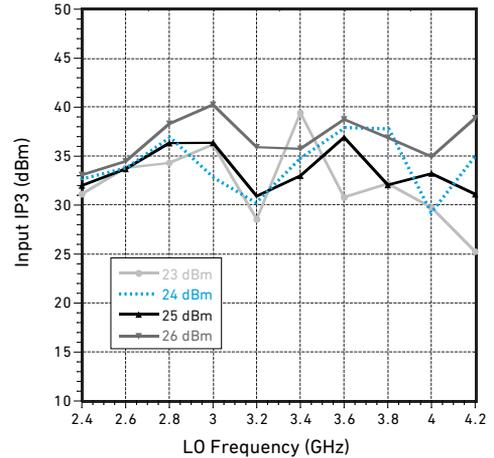
Figure 4. Input IP3 for S-band GaN mixer. IF=100 MHz USB.
