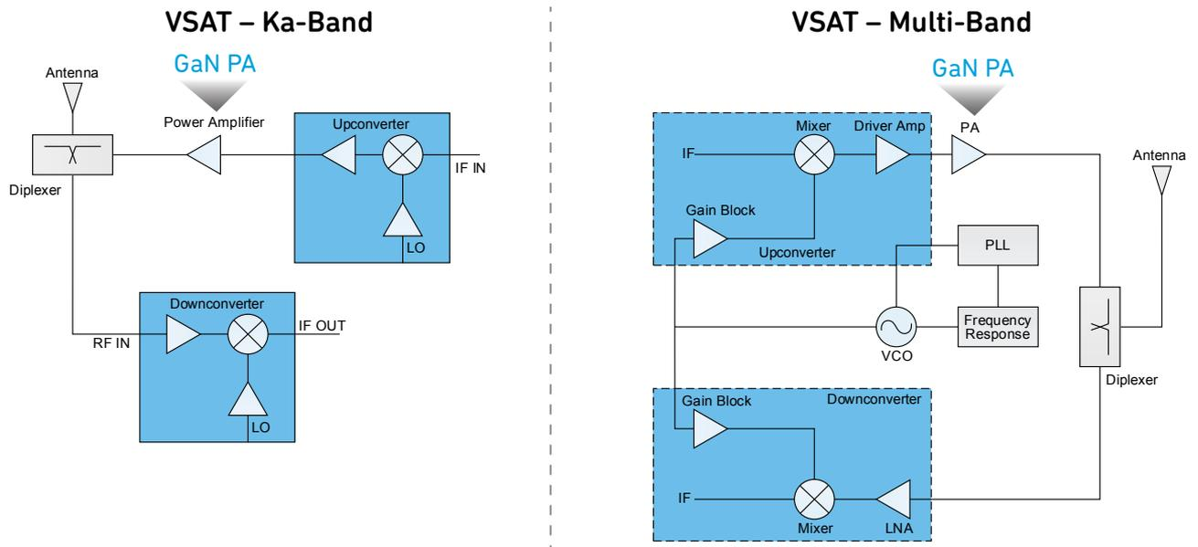
Figure 5. Satellite terminal system, VSAT block diagrams.
