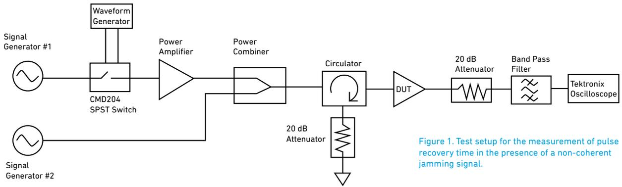
Figure 1. Test setup for the measurement of pulse recovery time in the presence of a non-coherent jamming signal.
