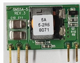
2.5V DC – DC Converter (for Gen2 AiP)
