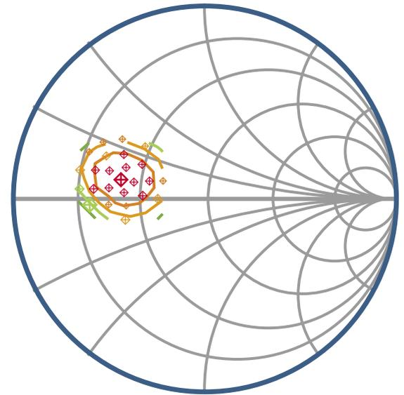
Figure 3c—Iso Pout Contours Simulated @ 1.85 GHz
