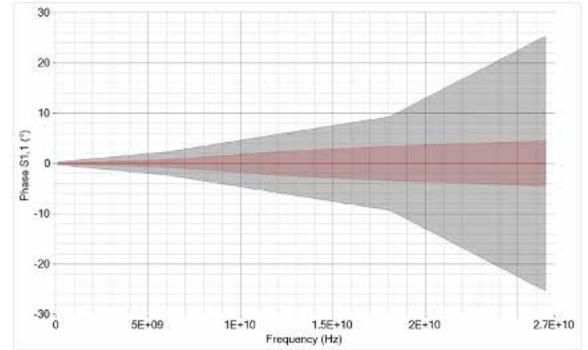
*S11\_phase measured on a short circuit termination
