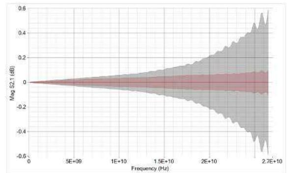
*S21\_mag measured on a short circuit termination
