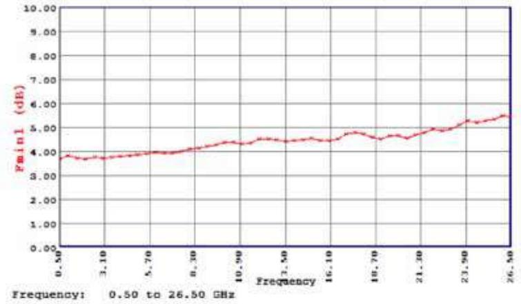
Figure 3. Typical Noise Receiver Calibration Using MT7553A03
