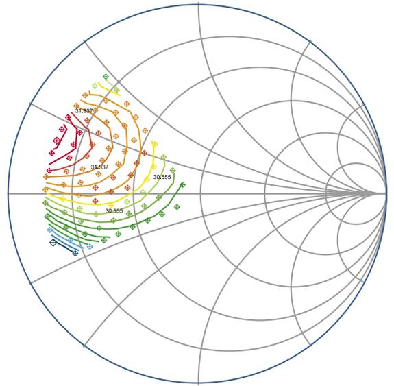
Figure 3b—Iso Pout Contours Measured @ 1.85 GHz
