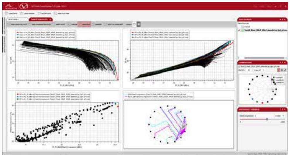
Harmonic-frequency high-speed load pull of 1 Fo impedance state, 16 2Fo impedance states, 16 3Fo impedance states and power sweep at 17 power levels for a total of 4352 measurement states in 15 minutes.
