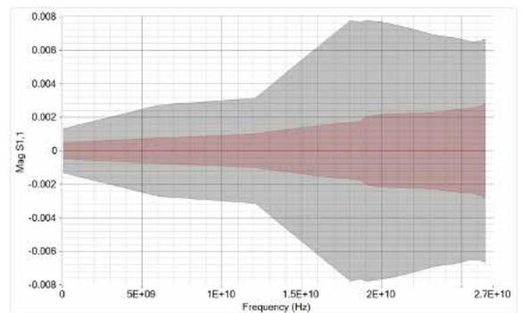
*S11\_mag measured on a 50Ω termination
