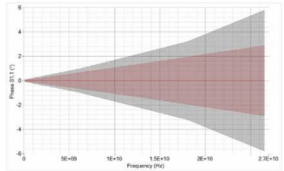
*S11\_phase measured on a short circuit termination
