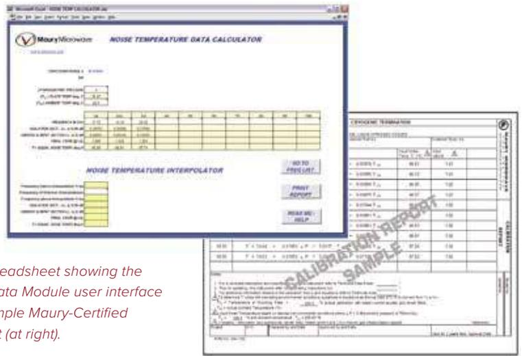
Typical Excel® spreadsheet showing the MT7250 Swept Data Module user interface (above) and a sample Maury-Certified Calibration Report (at right).
