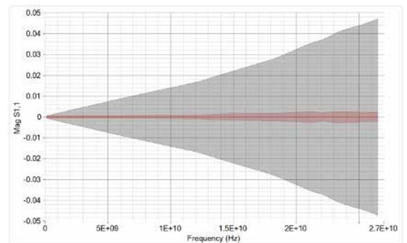
*S11\_mag measured on a short circuit termination
