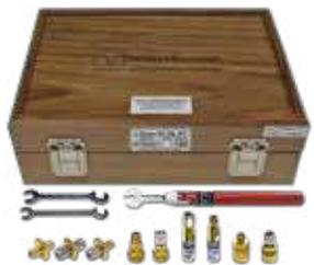
Maury precision 2.92mm VNA calibration kits include each of the calibration standards and tools shown in the tables at the right. The 8770CK40/50 kits do not include adapters; the 8770CK41/51 kits include one each of the in-series adapters shown. Other in-series and between-series adapters are sold separately.
