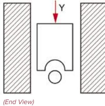
The probes used in slide-screw tuners are wideband in nature, and have similar reflective properties over a wide range of frequencies. In order to increase the overall useful bandwidth of the tuner, two probes of varying dimensions are independently used within a tuner; one for low frequencies and one for high frequencies. In this manner, it is common for slide-screw tuners to achieve an overall frequency range of several octaves to over a decade.
