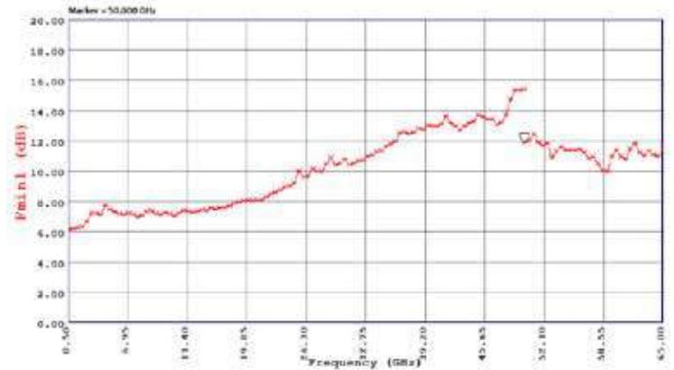
Figure 5. Typical Noise Receiver Calibration Using MT7553C01
