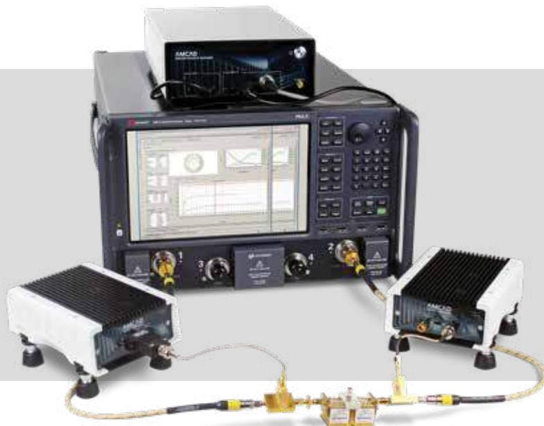
Active load pull replaces passive tuners at one or more frequencies with “active tuners”, which use a magnitude and phase controllable source to inject power into the output of the DUT, thereby creating the “reflection” signal needed to vary the impedance presented. Active load pull overcomes the mechanical and VSWR challenges presented by harmonic passive tuners, as well as tuning isolation challenges between the different frequencies related to the combined movement of the tuner’s slugs.
