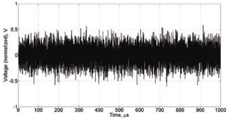
Figure 8 Time-domain representation of an LTE signal
