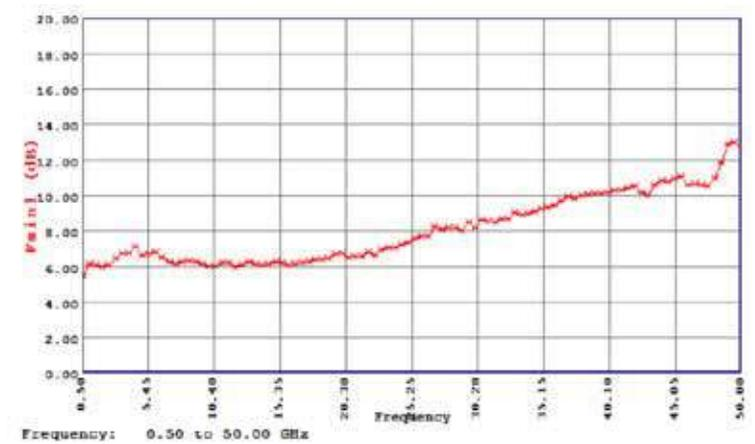
Figure 4. Typical Noise Receiver Calibration Using MT7553B03
