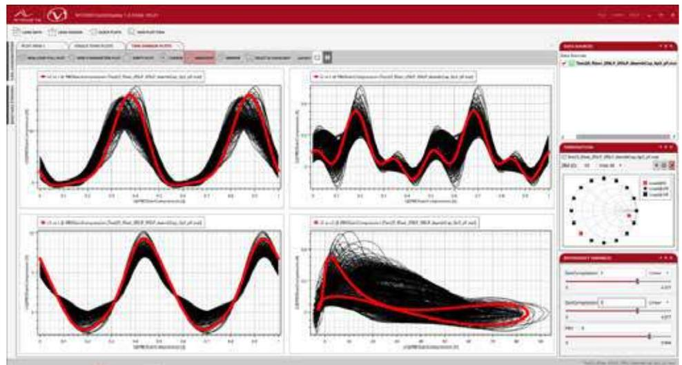
Harmonic-frequency high-speed load pull of 1  $F_0$  impedance state, 16  $2F_0$  impedance states, 16  $3F_0$  impedance states and power sweep at 17 power levels for a total of 4352 measurement states in 15 minutes, with the addition of NVNA time-domain voltage and current waveforms and load lines.
