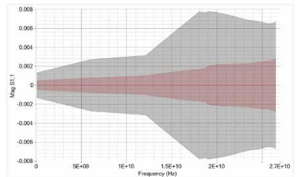
*S11\_mag measured on a 50Ω termination
