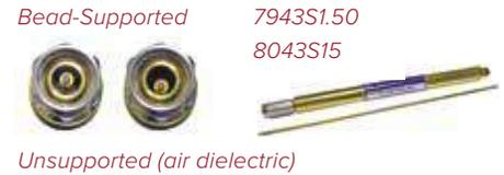
better impedance and electrical length accuracies, as well as lower VSWR (the center conductor floats free in the air line body, and the male connector nut is retractable to facilitate insertion of the center conductor contact before the thread-on connection tightened.
