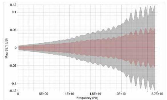
*S21\_mag measured on an airline
