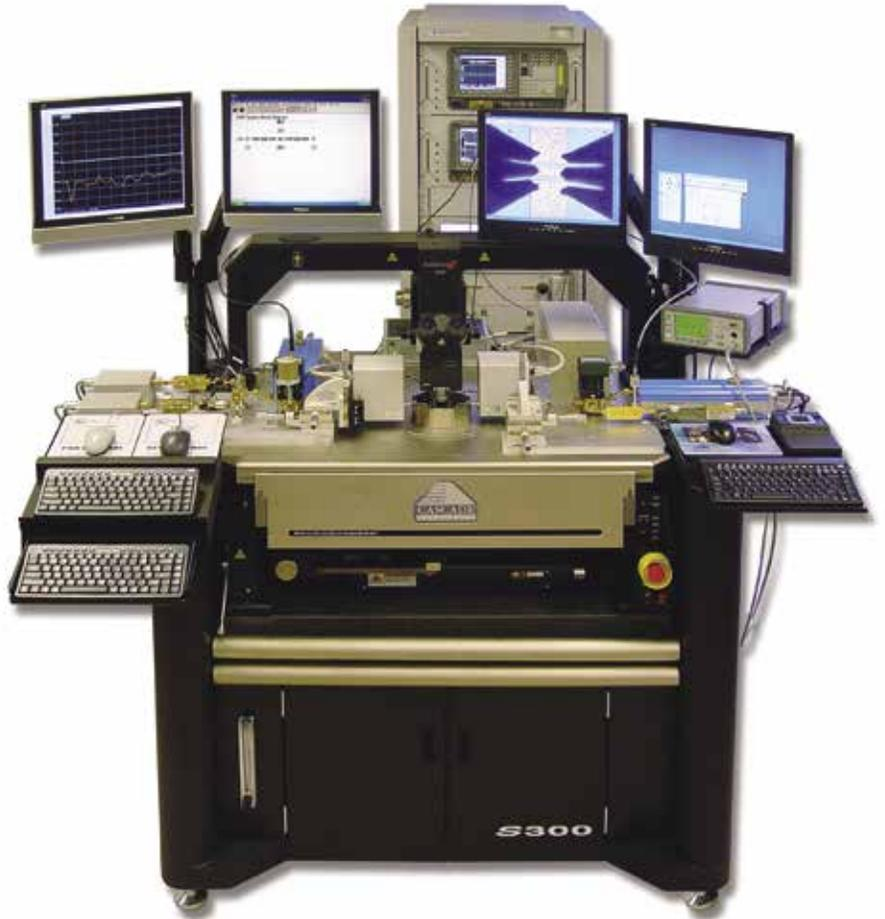
*MT900-series integrated on-wafer millimeter-wave s-parameters, noise parameters and load pull measurement system.*
