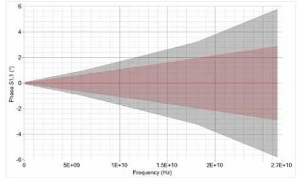
*S11\_phase measured on a short circuit termination
