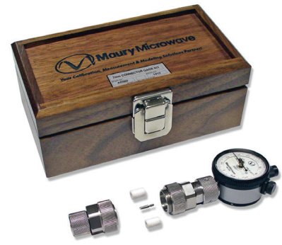
A028D – 7mm analog connector gage kit
