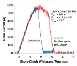
Critical to prevent failures like motor short circuit where the FET faces full voltage (V<sub>DD</sub>) in ON-state.
