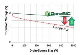
GeneSiC packaged and bare-die FETs can be paralleled reliably for high-power applications
