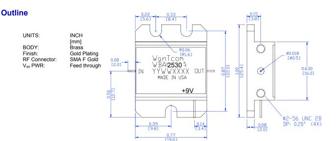
!!Warning: Only use 3/16" long #2-56 screws to mount the SMA connectors. Longer screw may damage the internal components.
