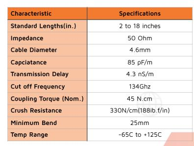
ConductRF 1.0mm Flexible VNA Test Cables are a proven solution for quality stable testing up to These cables have a minimum bend of 25mm(1.0"). Each assembly is serialized and supplied in a protective tube with test data.
