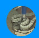
Induction Soldering LSA Cables are all terminated with Direct Solder style connectors for higher RF performance.
