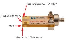
SIGNAL MICROWAVE 2" Microstrip on 5 mil ISOLA ASTRA MT77 with FR-4 Backe \* 1" Grounded Coplanar Waveguide (GCPW) on 5 mil ISOLA ASTRA MT77 with FR-4 Backet SIGNAL 2" Grounded Coplanar Waveguide (GCPW) on 5 mil ISOLA ASTRA MT77 with FR-4 Backe
