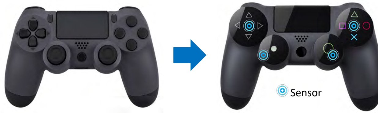
Traditional design of drone controller can be upgraded with touch-sensitive Qorvo HMI force sensor
